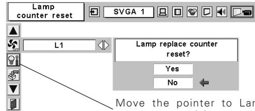
Move the pointer to Lamp counter reset and then press the SELECT button. The message "Lamp replace counter Reset?" is displayed.
