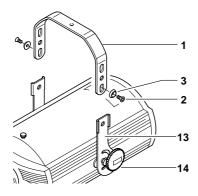
The bracket (1) can also be fitted towards the bottom of the projector. To do this, it is necessary to extract the knobs (14) from the rear hole and turn through 180° both the plates (13) and the spacers (15), then re-insert the knobs (14) into the front hole.
